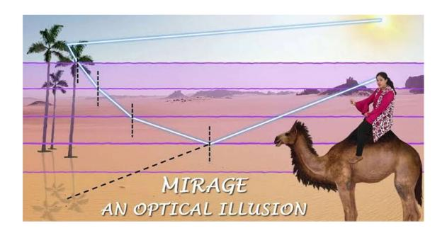
To a distant observer, the light appears to be coming from somewhere below the ground. The observer naturally assumes that light is being reflected from the ground, say, by a pool of water near the tall object.
